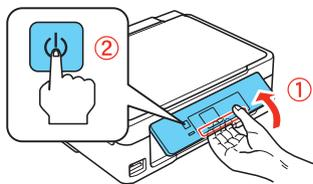
**Note:** If you want to lower the control panel, squeeze the release bar underneath.
