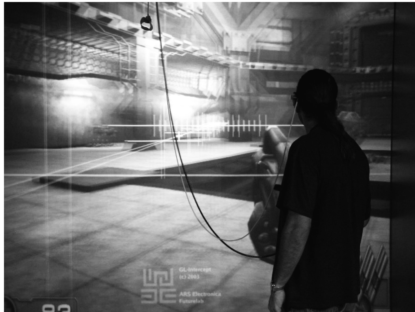
Figure 4: VRizer showing UT2003 in the ARSBOX on four walls with head tracking, wand bindings and softgenlock
