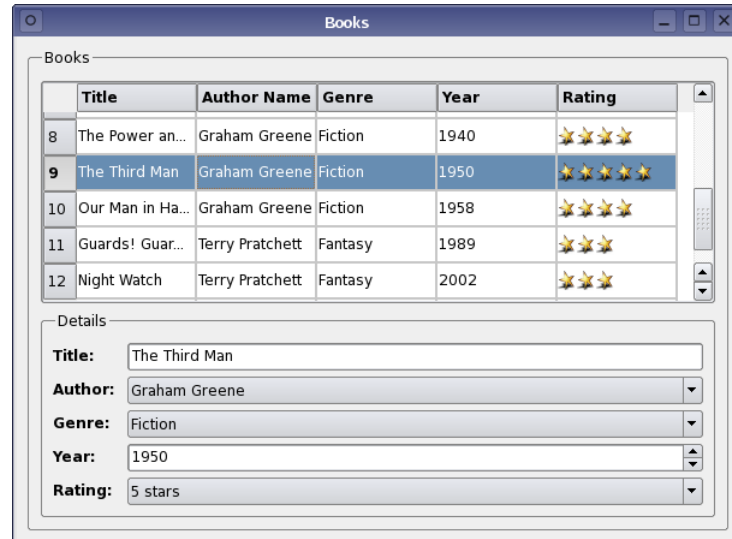
Figure 20: The Qt 4 Books demonstration shows the integration between Qt's SQL classes and the model/view framework.
