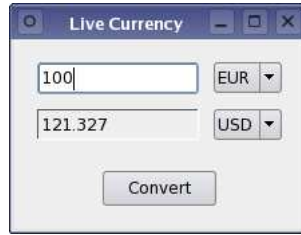
Figure 28: A live currency converter that uses the QTcpSocket class to send and receive data from a remote server.
